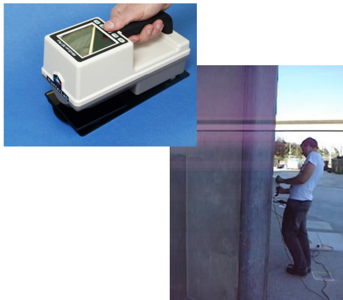
Figure 7. Measuring tonal variance of coloured precast concrete at hotel, Brisbane Airport, using HunterLab MiniScan Spectrophotometer.
